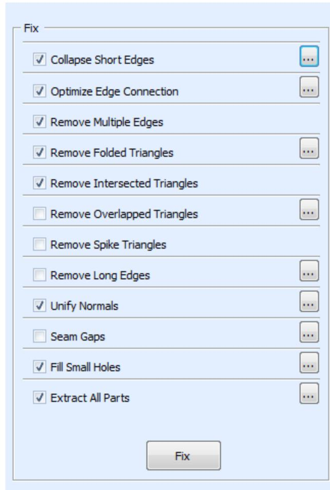
Click on one of the right side buttons
