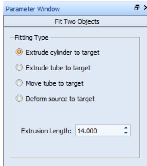
9. **Fit Tube to Template:** This step uses the **Fit Two Objects** command to extrude each tube up and down, or only extrude down if the *Fixed Top* option is selected. In this example, we checked the *Fixed Top* option and set the *Extrusion Length* to -0.1 mm measured from the end cap of a tube to the template surface. The result is shown below:
