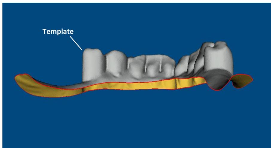
6. **Fill Boundary by Skin on Template:** This step uses the **Fill Boundary by Skin** command
