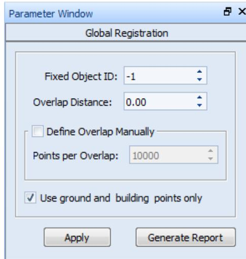
Once the registration process is done, Press the [Generate Report] button to export the result to a PDF file. You can view the improvement of mean and stand deviation on each strip and the total improvement after adjustment. The registration report is shown below:
